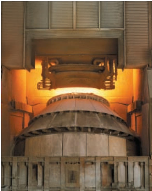
A basic oxygen furnace converter in operation
