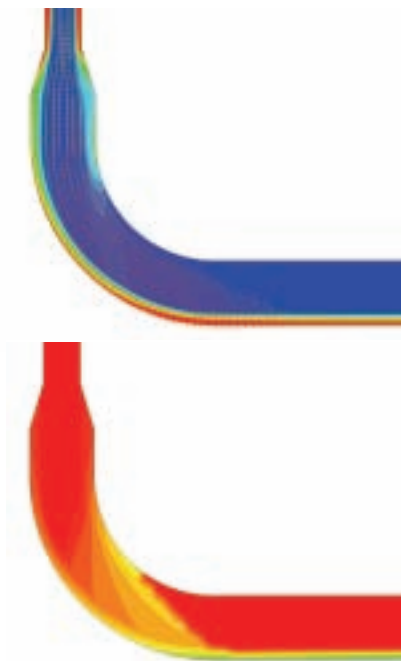
Contours of the solid phase volume fraction with solid phase velocity vectors (left), and Sauter mean diameter (right) in the vicinity of the bend for an inlet jet pressure of 1.5 barg, inlet gas velocity of 30 m/s, average inlet granule diameter of 57.8 \mu\text{m} and granular material density of 1200 \text{kg}/\text{m}^3 . The results show the solids collecting near the outer wall of the bend and lowering the Sauter mean diameter because of increased attrition.
