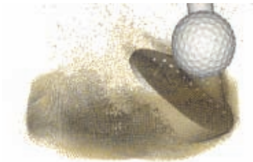
Close up of a golf ball deforming after being struck in a fluid structure interaction simulation, computed using ANSYS AUTODYN software
