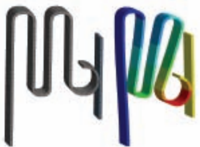
FEA simulations, such as the spring plate shown here, take into account factors such as contact between components and loading in order to predict displacement. The initial mesh is shown on the left while the contour plot on the right depicts displacement.
