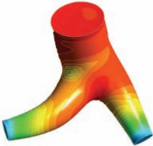
Contours of pressure on the vessel walls at peak systole
