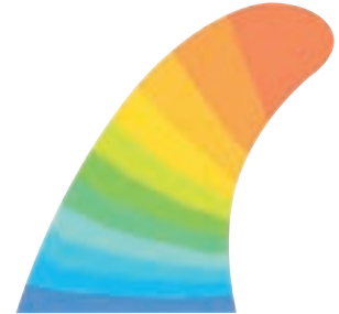
A finite element analysis is used to compute the deformation on the fin, illustrated here as displacement magnitude, the major component being the displacement in the z-direction (into the page).
