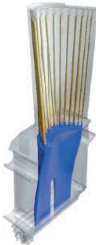
The internal features of the blade geometry include the plenum (blue) and the cooling channels (gold).
