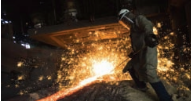
Man standing beside the pig iron channel, adjacent to where the hot metal flows
