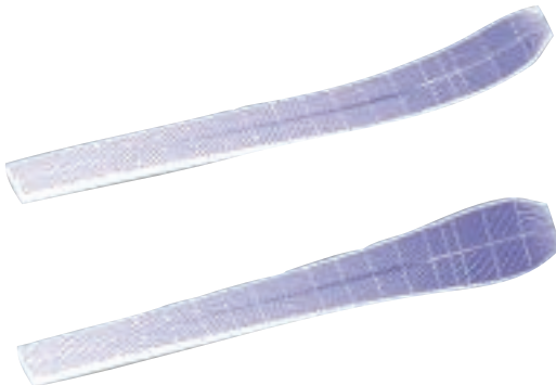
Images generated by FEA for (top) the second flexural mode of the front part of a ski and (bottom) the first torsional mode
