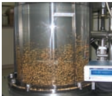
Solids distribution in a stirred tank driven by a standard PBT (left) is compared to that in the same tank driven by the optimized impeller (right); the cloud height is greater when the optimized impeller is used because the solids that collect under the PBT impeller are more uniformly distributed.
