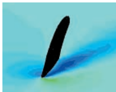
Contours of dynamic pressure on a plane slicing through the fin
