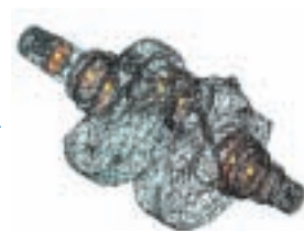
The ANSYS model generated by ANSYS Workbench to obtain the Modal Neutral File
