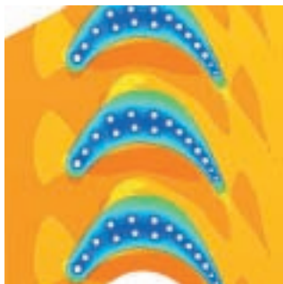
Temperature contours in the flow field and through the blade at a radial location near the blade platform (left) and outer casing (right)
